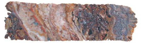
Photo 10.4 - P1 Lolon Vein in drill hole CHAG-03, 104.5m.
