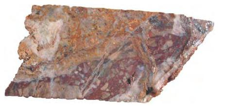
Photo 10.4 - P3 Lolon vein in drill hole CHAG-05, 39.4 meters.
