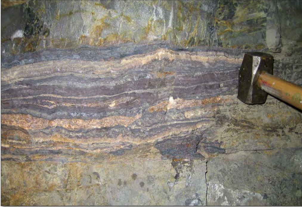
Figure 7-8 Photograph of Banded Sphalerite-Wurtzite (schalenblende), Pyrrhotite, Stannite, possible Cassiterite and Ag sulfosalts, No.3 Vein, Chocaya (Oploca) mine.
